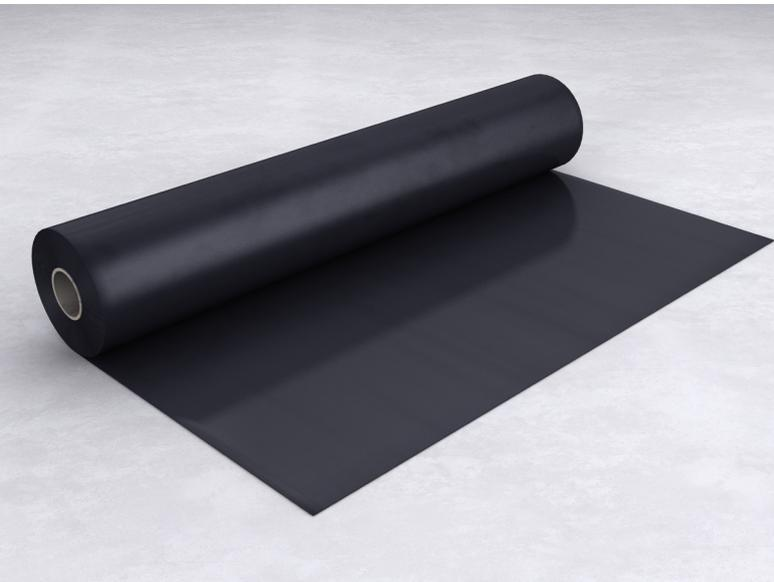
The Cordek Gas Resistant DPC is a polymeric DPC, designed for use in applications where combined damp proofing and gas protection is required. The DPC is robust and flexible, performing well under high compressive loads.
