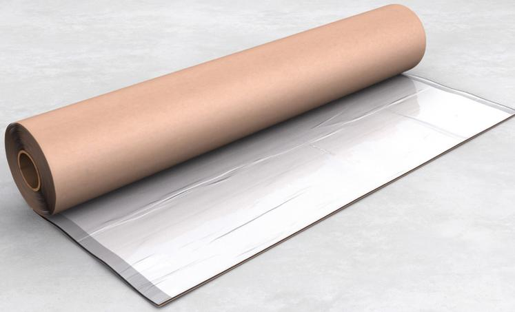
The Cordek Gas Resistant Self Adhesive Membrane is generally used within foundation construction, predominantly to prevent the transmission of ground gases in both horizontal and vertical applications. It is manufactured using an aluminium/polythene laminate coated on one surface, with an additional layer of self-adhesive polymer modified bitumen.
