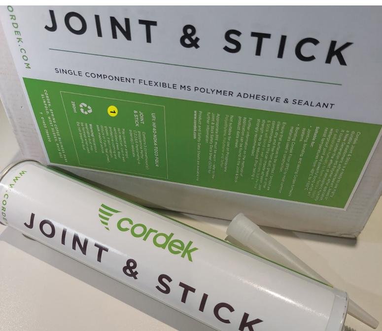
Joint & Stick is used to bond Cordek Filcor (EPS) to most common materials used in construction and for fixing, jointing, and sealing Cordek formwork systems.
