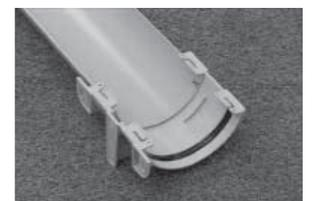
The notched gutter end is located under the notch adaptor and the joint completed by clipping the gutter under the easyclip on the front of the fitting.
