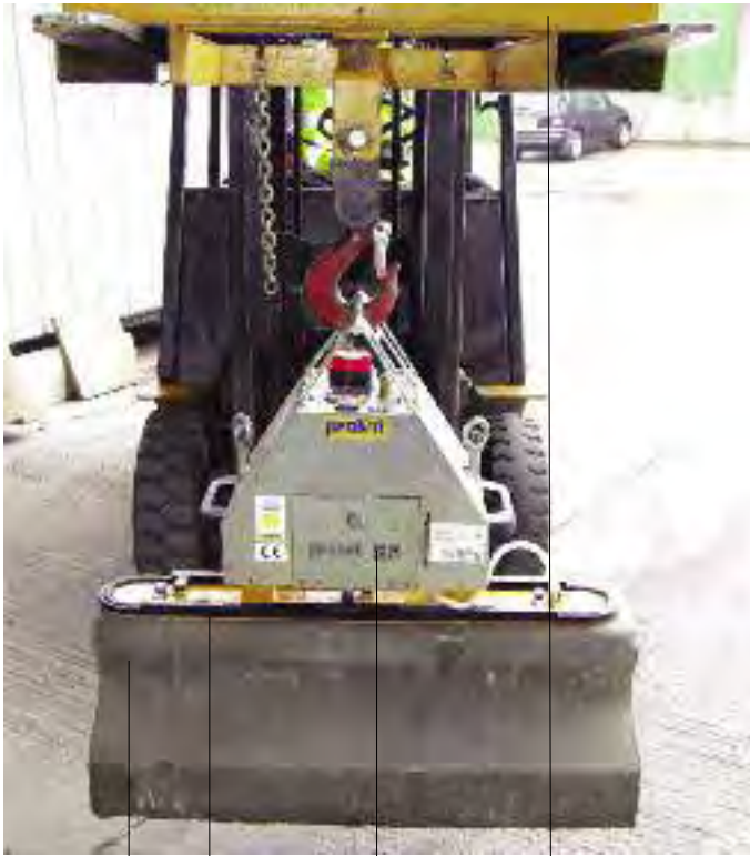
Trief Cadet Kerb unit 220kg Vacuum pad SWL 350kg Vacuum lifter SWL 500kg Fork Sleeves with Lifting Hook SWL 2500kg
