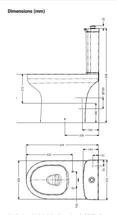
Navlin Standard-Height Close-Coupled Toilet Pan & Cistern with Raised Push Button Flush
