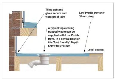
Please Note: Trays are shown in colour for illustrative purposes only. Low profile trays are not designed for use with pumped wastes.
