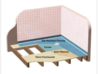
Tuff Form® offers superior strength and rigidity which can support a bath and bather. Installed with a Bath-to-Tray Adaptor, this provides an easy upgrade from a conventional bathroom to a wet floor showering area when needed.
