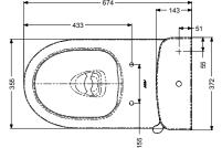
Navlin Raised-Height Close-Coupled Toilet Pan & Cistern with Lever Flush
