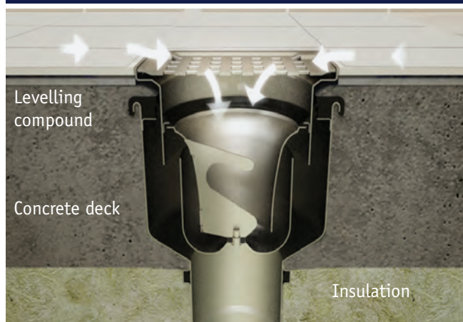
Concrete and tiles without membrane
