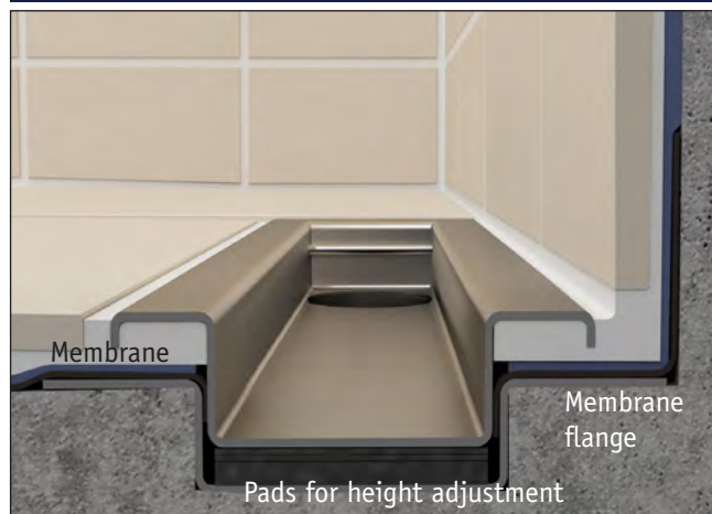
Tiles and liquid membrane
