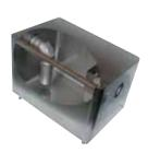
BLUCHER Grease separators - A range of standard size grease separators for installation either above or below ground. The BLUCHER grease separators have been designed to work with dosing units (also supplied) which treat the separator with bacteria that digests the grease. This means little maintenance is required but, unlike direct dosing systems, allows for failsafe grease storage should the dosing be negated.
