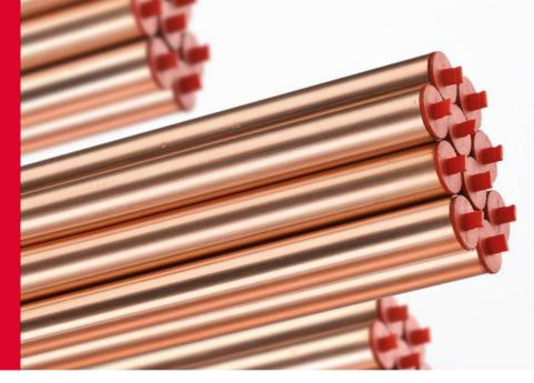
Yorkshire Medical Gas Tubes are specially cleaned and packed to ensure they are suitable for medical gases and/or vacuum lines. In oxygen lines, spontaneous combustion can take place with any greases or hydrocarbons in the tube, and the cleaning process eliminates this risk. Additionally, the cleaning takes away malodour from any residual lubricants that may taint breathable gases.
