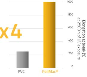
ISO 4892-3 "Plastics - Methods of exposure to laboratory light sources (Fluorescent UV lamps)" ISO 527-1"Determination of Tensile Properties"
