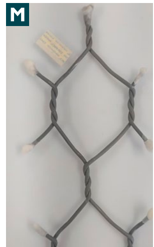
Test Specimen, before and after Salt Spray Test (ISO 9227)
