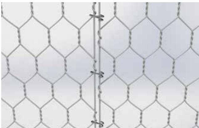
Simple offset panel to panel connection
