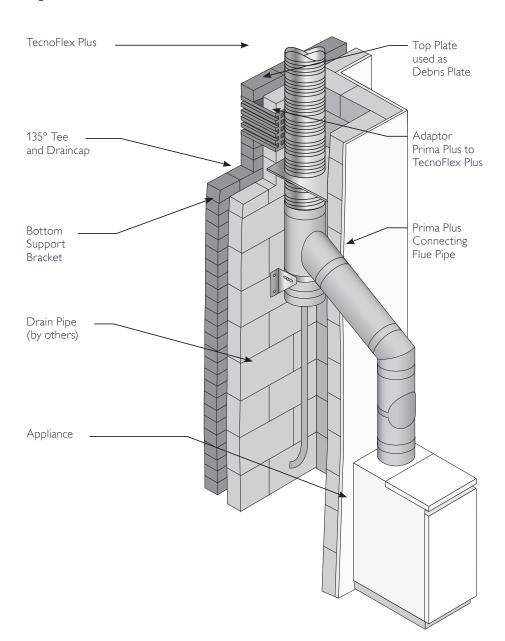
Fig. 1 TYPICAL CONDENSING APPLIANCE CONNECTION
