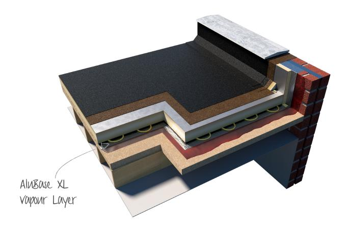
A self-adhesive bituminous waterproofing membrane that forms a barrier against vapour and gases.
