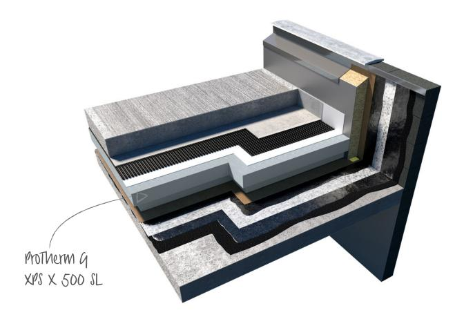
A rigid, closed cell type extruded polystyrene board with integral high density skin.
