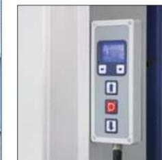
Display unit in a small box placed at the side frame.
