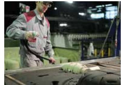
Insertion of the sand core
