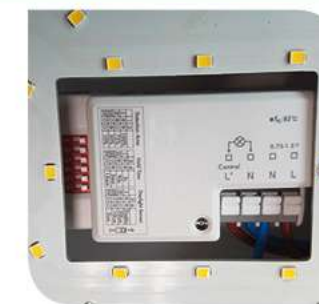
Quick and simple adjustment of 'Time ON', 'Light Level (LUX)' and 'Sensitivity' control settings.
