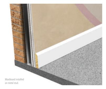
Maxiboard can be installed on an independent metal stud in front of a masonry wall construction to exceed the acoustic requirements of Part E of the Building Regulations or to significantly improve domestic comfort / privacy. The installation guidance below refers to the use of 50mm wide Protektor Eco tracks and studs but please note that other manufacturers are available.
