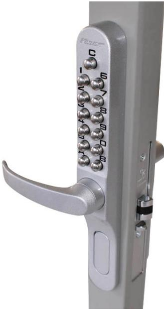
The narrow stile Keylex 700AR design, with its built-in clutch mechanism protecting the lock furniture, will suit stile widths down to 45mm in this configuration and is particularly suited for use on aluminium and hollow metal door sections. The Keylex 700AR can be expected to give many years' service if specified and maintained correctly.
