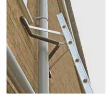
The Ladder Stand Off features a large V which allows the ladder to span around down pipes or rest on corners of buildings. The top of the ladder is kept 330mm off the wall making it ideal for use when working under eaves.
