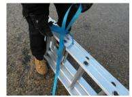
Tie the strap around the footing Ladder stile and the third rung of the Ladder
