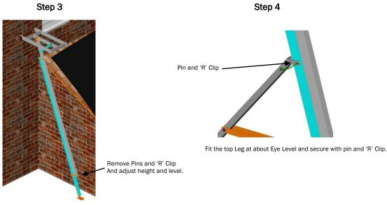
Position the Leg and frame against the wall and adjust for height and level.
