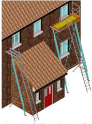
Make sure the Easi-Dec platform and the End support frame are Level. REMEMBER: The Catwalk will sit a minimum of 300mm on the 2m Dec and will completely sit over the End Support frame. Set the gap between the two with this in mind.
