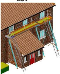
Raise the Cat walk as described in the 4.6m walkway assembly instructions sheet with details on how to install the Guardrail and toe boards.
