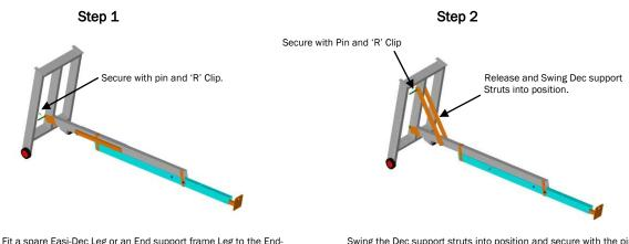
Fit a spare Easi-Dec Leg or an End support frame Leg to the End Support frame and ensure the Pins and 'R clips are secure.
