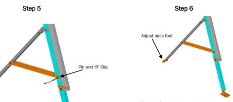
Swing the Brace into position and secure with the pins and 'R' Clips provided.
