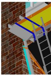
Ensure the Catwalk sits over the whole End Support Frame and Secure using the Two Ratchet straps Provided.
