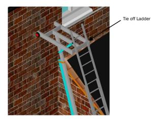
Tie off the frame securely to the building in positions indicated in step 11. Erect the Ladder against the End support frame and Tie
