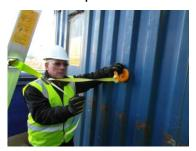
Keeping the strap horizontal attach the suction cup to a suitable glazed window. The above picture is for demonstration purposes only, usually the cup is positioned against the glass of a conservatory.
