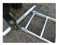
Push the stabiliser foot into the bottom of the footing Ladder.  $% \label{eq:ladder} % \label{eq:ladder}$
