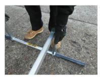
Slide the eaves batten over the stiles of the footing Ladder and locate using the captivated pins into the height adjustment holes of the stiles. Ensure the pins are pressed home fully.
