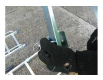
Remove the pins from the Eaves batten.
