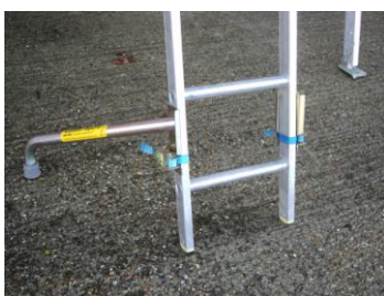
Use Ladder spurs supplied by Easi-Dec to aid stability and prevent outward slip.
