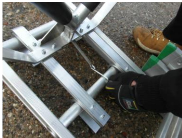
Pull the sprung hook over the second rung ensuring it's firmly fixed into position. WARNING! It is very important this sprung hook is fixed into position before use, as it prevents the Ladder stand-off sliding off the top end of the Ladder.
