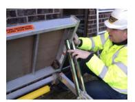
Swing the Dec support struts and secure with the Pins and 'R' Clips provided.
