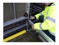
Fit both Legs using the Pins and 'R' Clips provided and ensure that the Pins are inserted outside in, to minimise the risk of the 'R' Clips being Knocked out. *REMEMBER:* Fit the Legs to the 'Normal use' hole Labelled on the underside of the platform.
