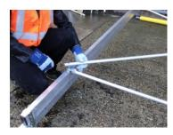
Swing out each Brace over to the opposite Leg and secure onto the retaining stud using the two 'R' clips provided in a downward position.
