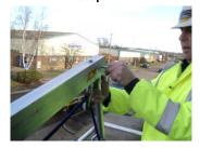
To fit the Support Tubes remove the Locking Pin from each end of the Lifting Beam, insert the Support Tube into the large hole on the underside of the Lifting Beam and replace the Locking Pin to
