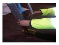
The Feet maybe adjusted in 25mm increments but in extreme cases either Leg can be adjusted Independently. Fit Pin and 'R' Clip to secure.
