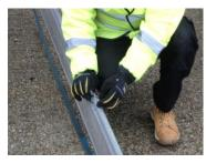
$\mbox{Pull}$  out the 'R' Clips and release the two Braces from their stowed position.
