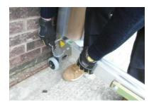
Fit both Legs using the Pins and 'R' Clips provided and ensure that the Pins are inserted outside in, to minimise the risk of the 'R' Clips being Knocked out. *REMEMBER:* Fit the Legs to the 'Normal use' hole Labelled on the underside of the platform.
