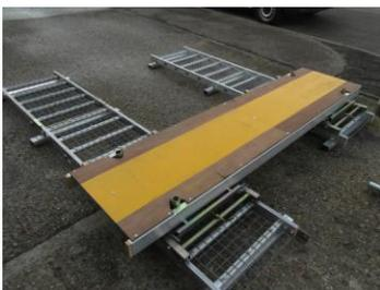
The Catwalk should be positioned uniformly over the trolleys.
