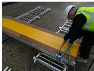
The Platform is now strapped to the trolleys with the ratchets straps provided. Repeat strap attachment for the second trolley.
