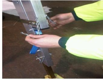
Adjust the height by removing the two Leg Pins and pulling on the Straps rolling the Solar Platform up the wall to the desired height and replace both Leg Pins remembering to also replace the safety 'R' Clips provided. After adjusting to height it will be necessary to re-level the Solar Platform by moving the feet either away or towards the wall.
