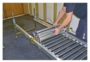
The Plasterer's Mate Low Level Safety Platform has been designed to allow low level interior work such as on walls and ceilings. The system overcomes the problems associated with traditional methods such as trestles and long boards by providing a quick and easy solution which can be simply rolled-up and carried under one arm.
