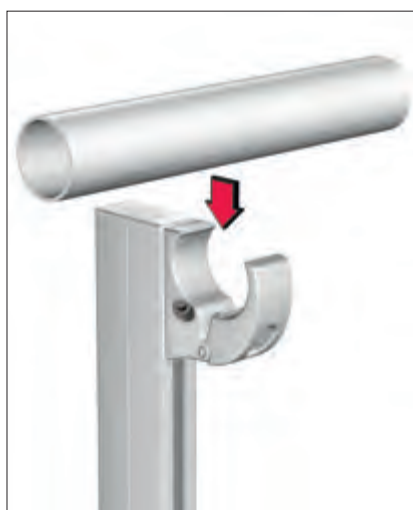
Positioning the rail
