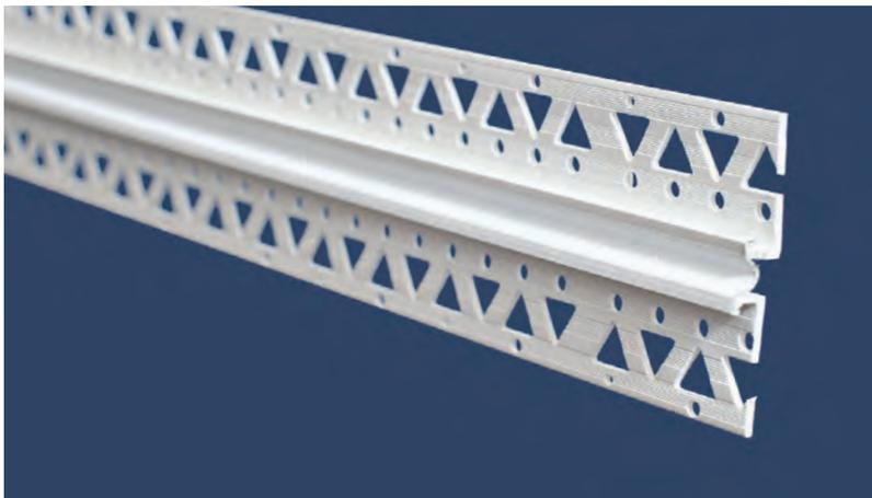
Protektor PVCu Movement Bead is installed vertically and used when providing a finished wall the facility to provide minor levels of Thermal movement within the rendered finish or were a day joint is required.
