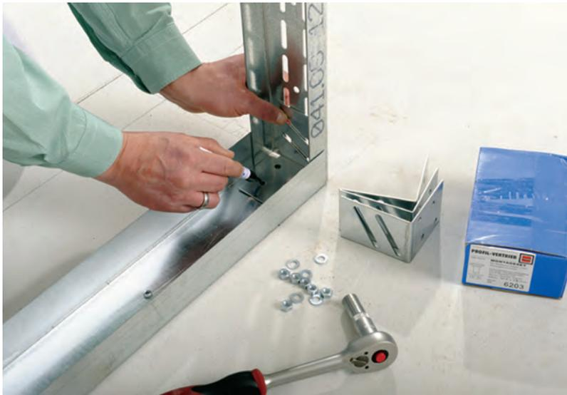
The Protektor Door Reinforcement system is designed to accommodate a range of door weights.
