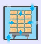
Vessel flooded under vacuum. The vacuum release enables the VACSOL preservative to penetrate into the timber cells under atmospheric pressure, in order to achieve a target penetration for the specified Use Class.
