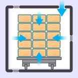
Venting of atmospheric pressure (second or 'double' vacuum) drives any surface preservative back into the timber cells. Timber surface drip dry.
