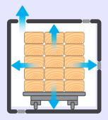
Vacuum created and timber cells evacuated of air.
