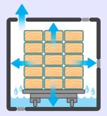
A second vacuum is applied to evacuate the timber cells of excess preservative. Timber surface wet.
