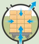
Cylinder flooded under vacuum with TANALITH wood preservative, with colour additive if required.
