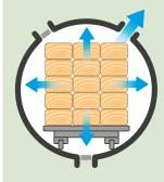
Timber loaded into treatment vessel. Initial vacuum applied and the timber cells are evacuated of air. Vacuum held.
