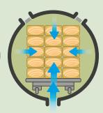
Hydraulic pressure is applied, enabling the preservative to penetrate into the timber structure, to achieve a target penetration for the specified Use Class.
