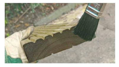
Timber which is rip sawn, equalised, planed or heavily sanded must be returned to the treatment plant for retreatment.
