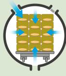
Low pressure inside timber draws in surface solution when vented to atmosphere. Treated timber is left to dry.
