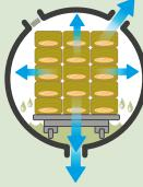
Final vacuum extracts excess preservative solution, which is pumped back to storage.
