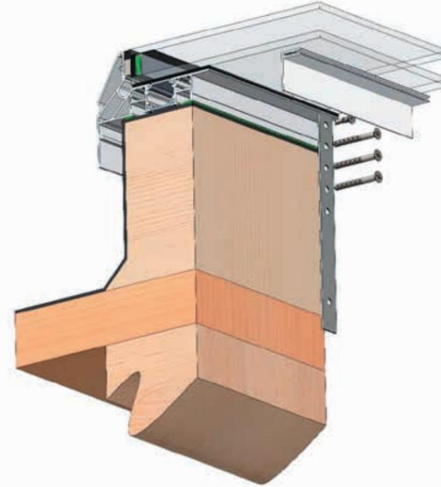
Locate top hole of FRL5601S-Fixing Plate to "V" groove on outer frame internal face and secure in place using FRL5603 4.8x16mm Self Drilling Screw 150mm away from each corner.
