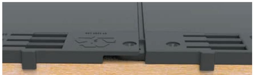
Each tile has two detachable nibs (F) at the top. These are used to hook the tile over the batten. When a batten has been fitted out of alignment or there has been some movement after fitting, the installer can break the nibs off as required if they find that the nibs no longer hook over the batten.
