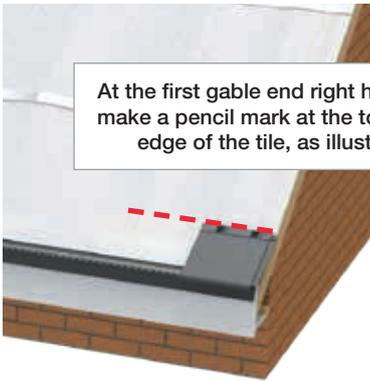
At the first gable end right hand rafter make a pencil mark at the top leading edge of the tile, as illustrated.
