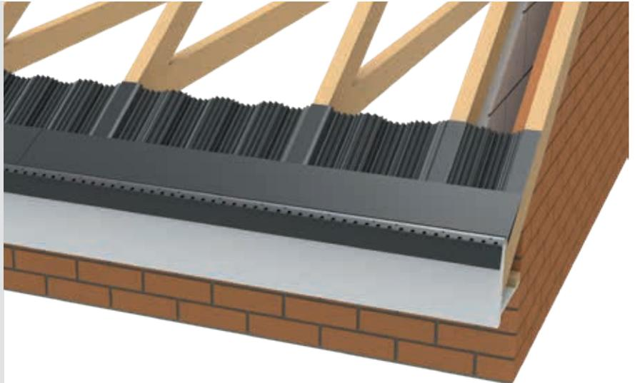
For abutment wall roofs ensure that the final Starter Rail located next to the wall provides a gap of 40mm away from the wall edge.
