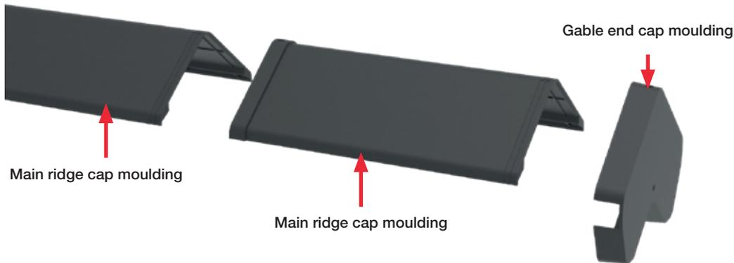
Starting at the right hand side of the roof, align and loosely fit the ridge cap mouldings over the ventilated ridge roll by interlocking the ridge sections together. At the gable the end cap envelopes the mitred dry verge before interlocking with the end ridge section (see illustration).
