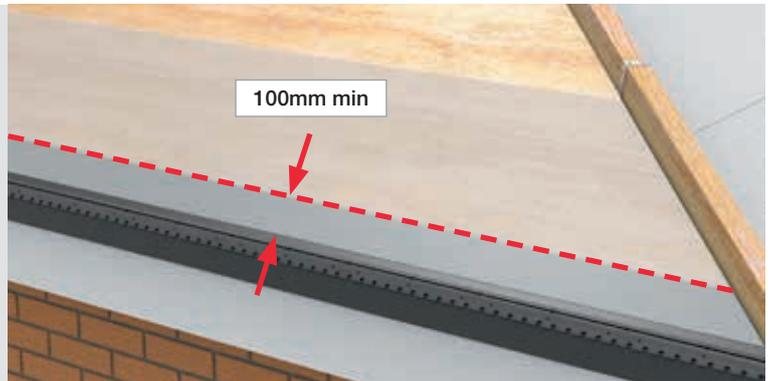
Starting at the right hand roof edge roll out and fix to the plywood roof panels EnvirolayFR® (ENVIROLAY) to the full roof face, fixing and securing the roof underlay at 450-600mm centres with clout nails as you go along. Overlap the universal eaves/support tray by a minimum distance of 100mm.
