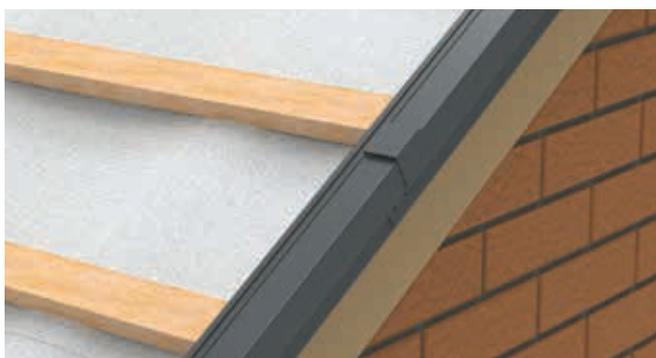
Fix a bracket clip, if required, with screw fixings ENVDVB, to join lengths of continuous dry fix verge when rafters are longer than 3m in length.
