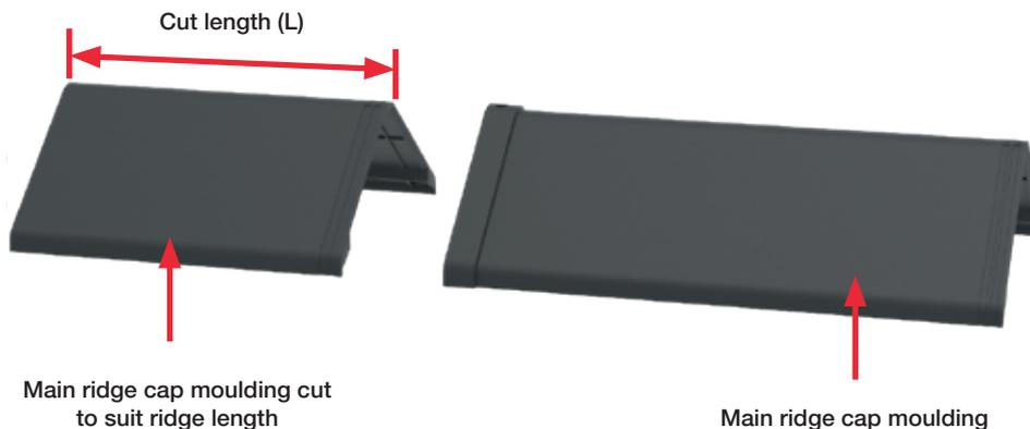
If the cut length (L) is less than half the length of the ridge cap moulding it is recommended that you cut two ridge cap mouldings and space accordingly.
