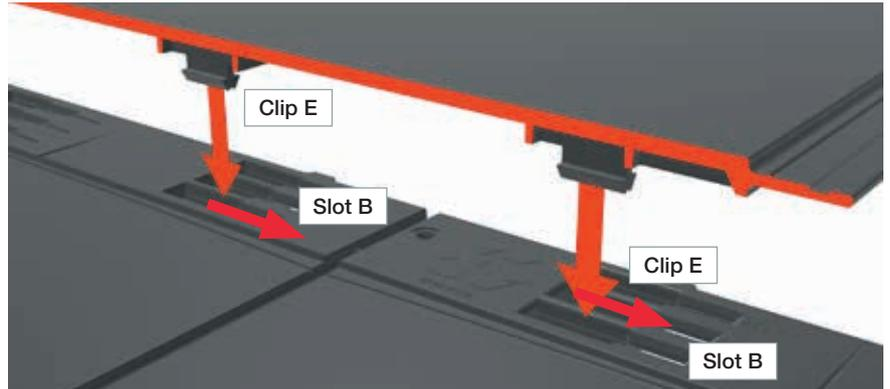
Envirotiles are clipped together using the two clips on the underside at the bottom of the tile (E) clipping into the slots at the top of the tile on the course below (B). Note that the tile must be aligned, then pushed down, then the tile is slid to the right to lock into the clip. The sliding action also locks the connecting strip into the adjacent tile slot.
