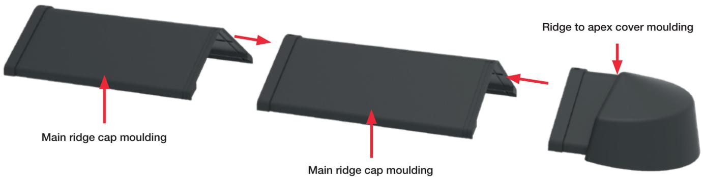
Starting at the right hand side loose fit the ridge to apex cover moulding over the hip to ridge apex. Then loose fit the ridge cap moulding over the ventilated ridge roll and then interlock with the next ridge cap.
