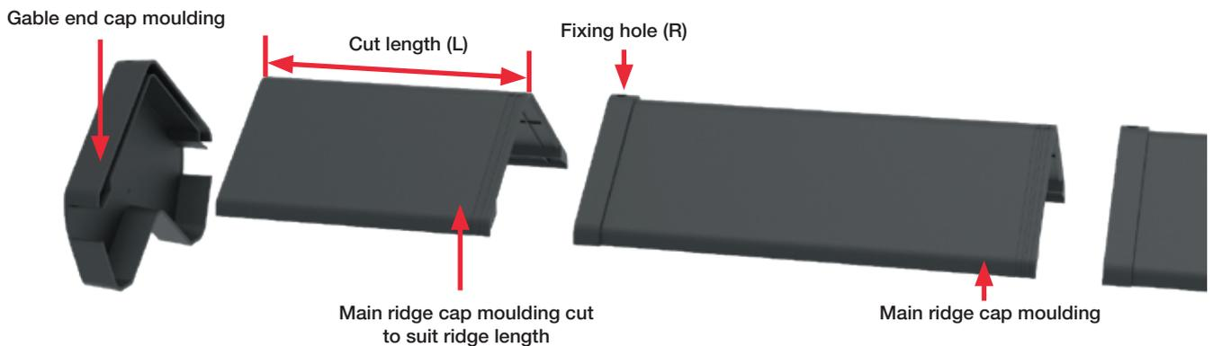
Lay out and interlock the main ridge sections together loosely along the full width of the roof. When correctly aligned permanently fix into place using the bedded batten as a fixture point for the 90mm x 6.3mm Stainless Steel Pozi Pan Self Tapping (ENVSCREW90) required to permanently fix two ridge sections together. Start the mechanical screw fixing procedure from the right hand gable end, using the fixing hole (R) on the apex at each end.
