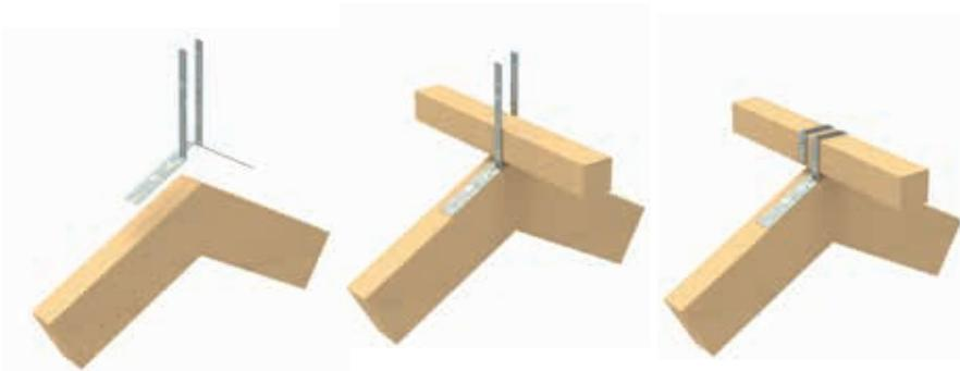
Note that the rafter straps are usually supplied flat and need to be bent to shape.
