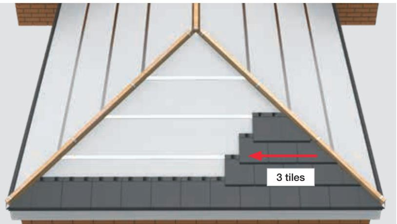
Continue fitting 3 tiles in stages until the roof is covered. On the left hand side ensure that you always fit a double tile on the hip angle. Trim the left hand tiles to the hip beam line, leaving a 20-25mm gap for ventilation and expansion.
