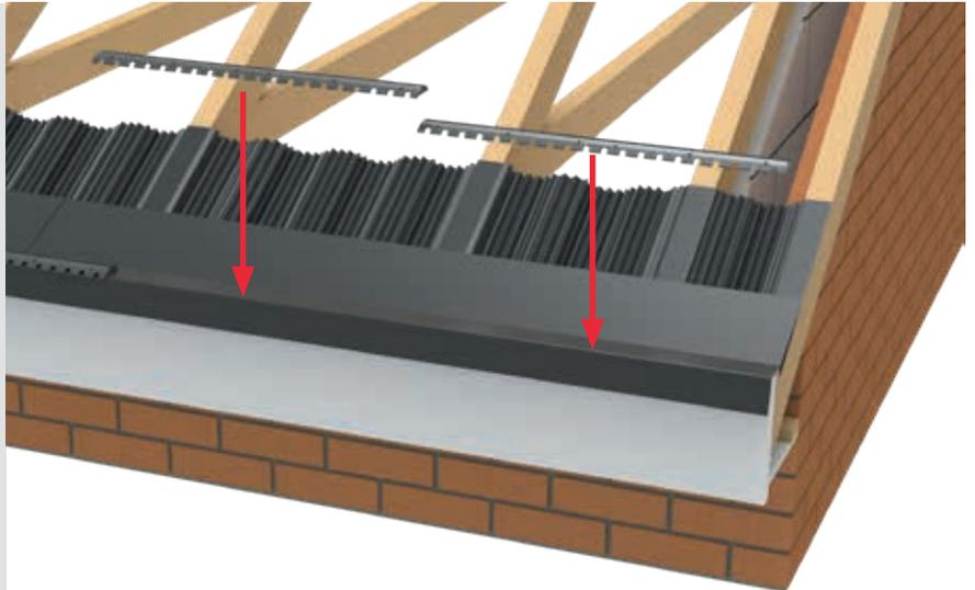
Starting at the right hand gable end verge, run through the full roof width with eaves bar/starter rails ENVEB then mechanically fix with stainless steel screws.
