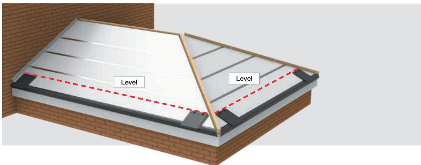
In a warm roof construction the Envirotiles are fixed directly onto the plywood roof face panels. There are no battens so it is very important that the installer checks that the first course line is level. The easiest way to do this is to clip a single tile into the starter rail at each end of each roof face and run a line as shown. Adjust the line so it is level - the starter rail allows for some tile adjustment.
