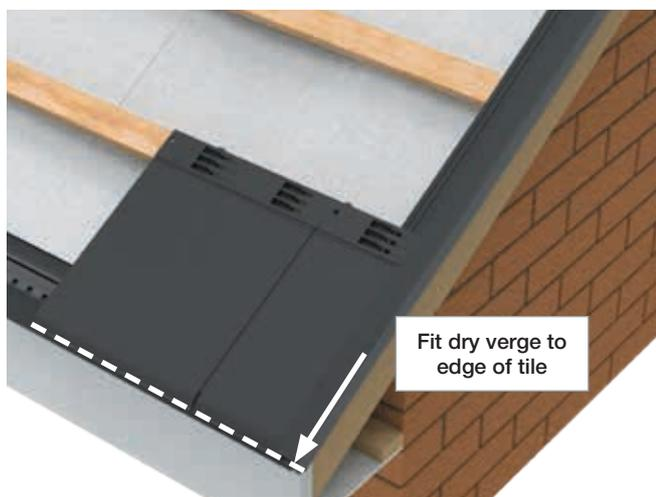
At the gable ends slide a roof tile (first roof tile) into the eaves/starter rail at the gable end as shown.
