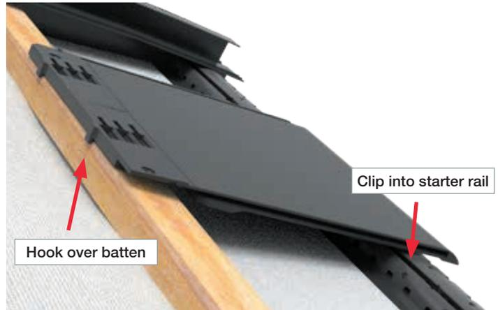
Use a full tile to start and cut off the right hand connecting strip.
