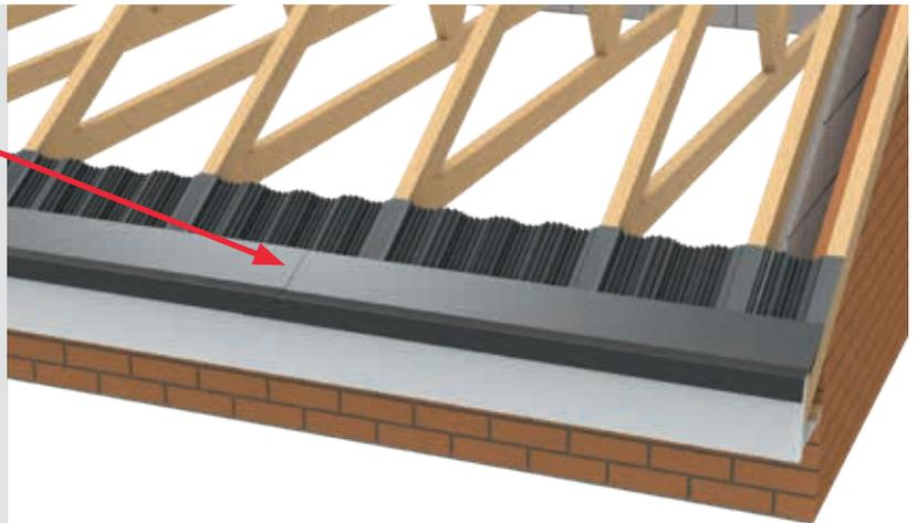
Butt up against the abutment wall with the felt support tray.
