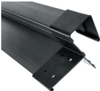
To finish gable ends it is recommended that the continuous dry fix verge (ENV3MDV) is used. This is fitted over the top of the battens and runs along the top edge of the end rafters at gable ends. Use dry verge brackets (ENVDVB) to join lengths of dry verge if required.
