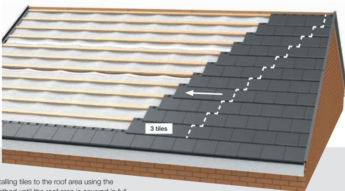
Continue installing tiles to the roof area using the 3 tile step method until the roof area is covered in full.
