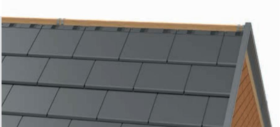
Place the ridge roll over the centre of the bedded batten and lay over the ridge apex ensuring the roof tiles are used as a substrate and overlapped by a minimum distance of 100mm either side of the apex.
