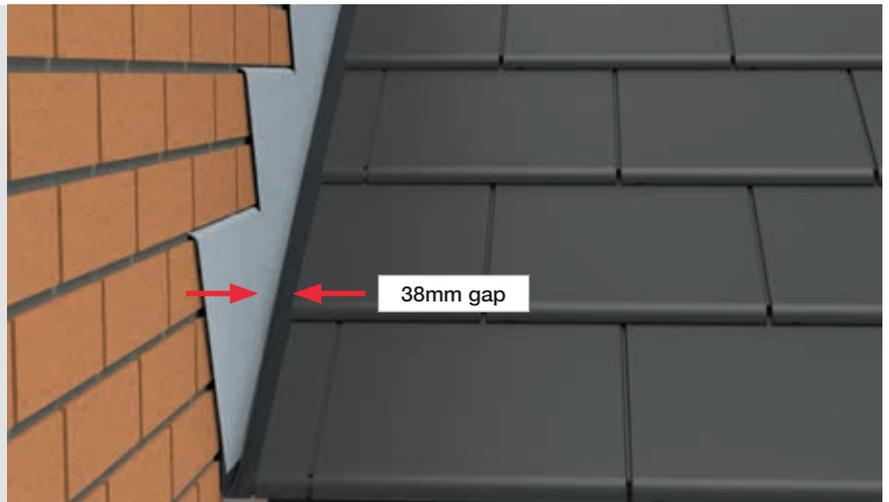
The 38mm gap between the parapet wall and roof tile edge provides the installer with enough room to engage the patented interlocking features into the surround tiles.
