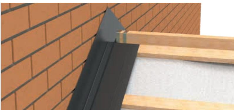
After fixing the abutment soaker correctly overlap/install the wall flashing to make watertight, as illustrated.
