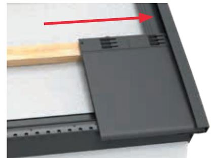
Take a new tile and clip into the starter rail, hook over the batten, then slide this tile into the end tile so that the connecting strip fits into the left hand slot of the tile. Push together ensuring there is a 5mm space between the top faces of the tiles.
