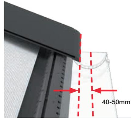
Note that the distance between the leading edge of the tile should be located approximately centre of the fixed gutter by a distance of 40-50mm.
