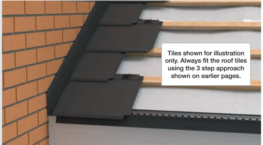
Leave a gap of 38mm between the abutment wall edge and end of roof tiles.
