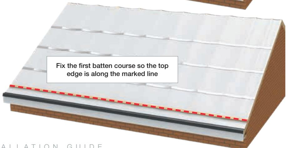
Fix the first batten course so the top edge is along the marked line
