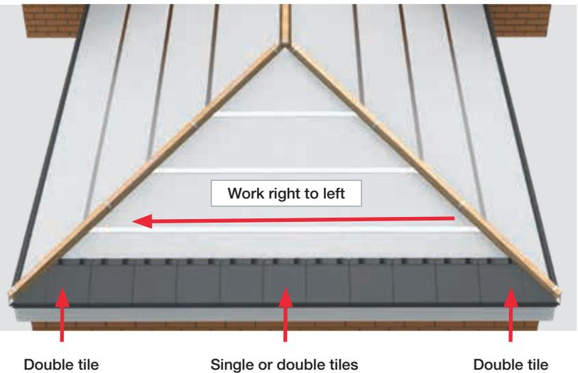
Using the same procedures detailed for gable wall roof types on page 24, working right to left along the roof face, fit 3 tiles at a time.
