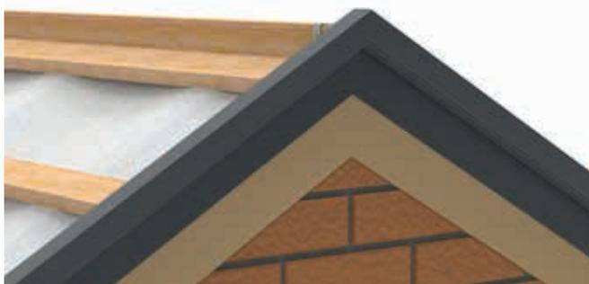
At the apex centre mitre cut and abut to the continuous dry verge unit to the correct pitch angle in readiness for the gable end cap to be fixed.
