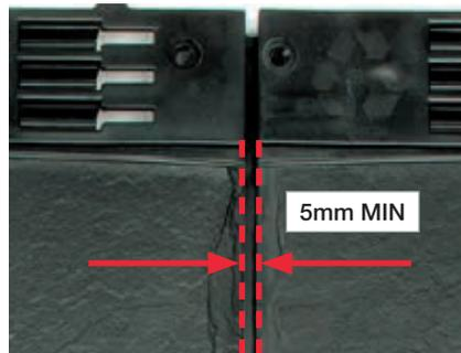
Note: An embossed 5mm marker/guide line is etched onto the tile interlocking insert fin to assist the installer with spacing.
