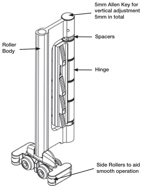
The double leaf roller incorporates a hinge which fixes the roller to the door sashes (top & bottom rollers) the rollers themselves have 10mm of adjustment (+ & - 5mm).
