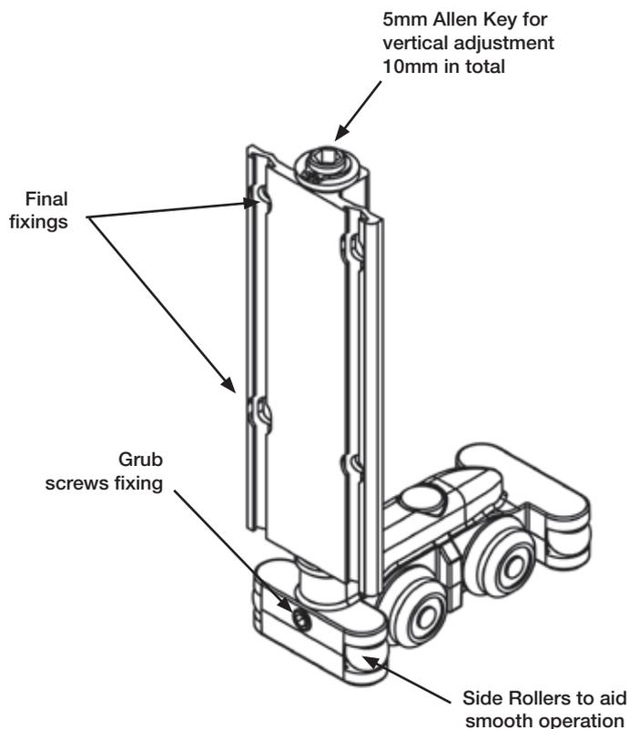
The single leaf roller is screwed directly in to the door sash euro-groove (top & bottom rollers) the rollers themselves have 10mm of adjustment (+&- 5mm).
