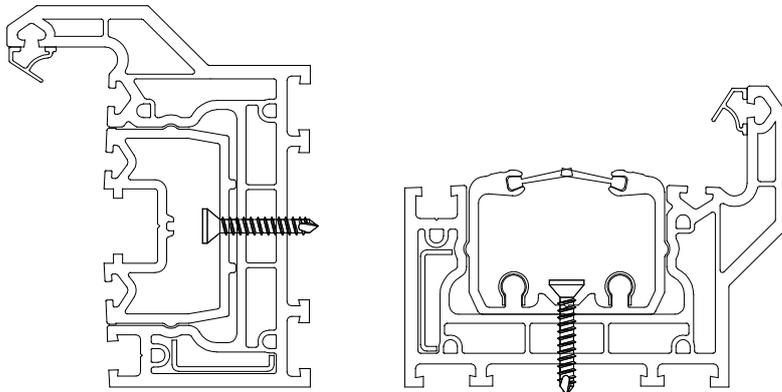
If this fixing is over tightened, it will distort the aluminium roller case and prevent the door from operating as it should. Fixings appropriate to the opening should be used.
