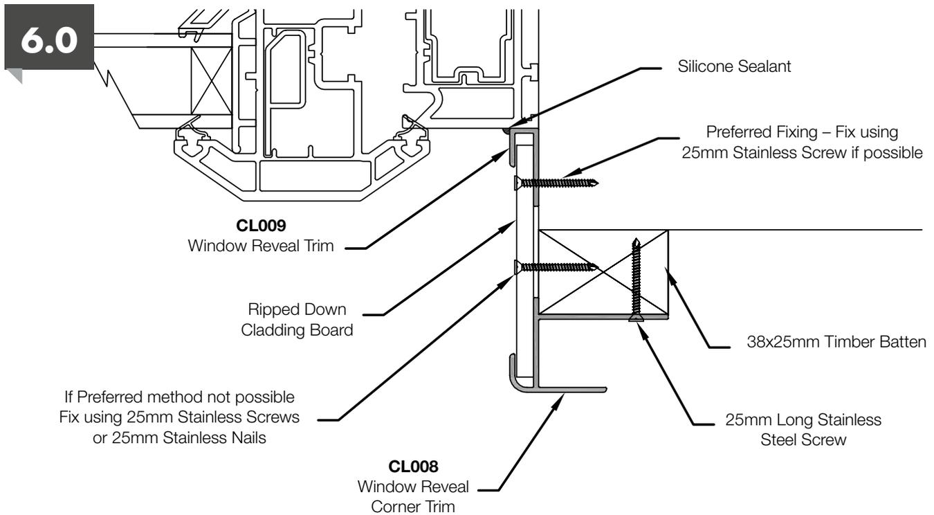
The Window Reveal Trims (CL008 & CL009) and Window Head Trims (CL003) need to be fitted before installation of the Cladding Board begins. This is to allow the trims to be fixed correctly.
