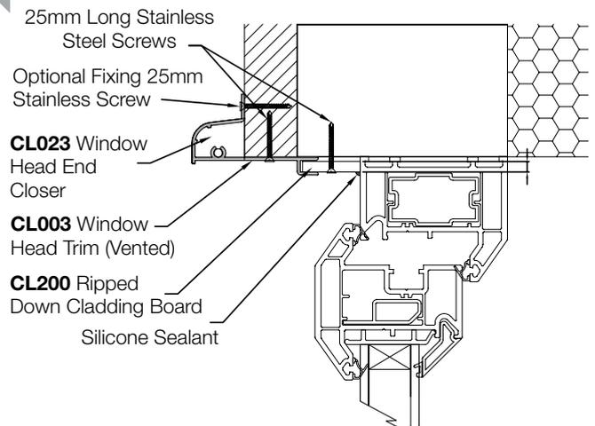
Cut down a section of Cladding Board to the required size. Position the board into the Window Head Trim (CL003) and fix head trim up into the timber battens using 25mm stainless screws. Once in position fix the board up into the brickwork and seal the end with a silicone sealant. (See page 12 for instructions on CL023 head end closer).
