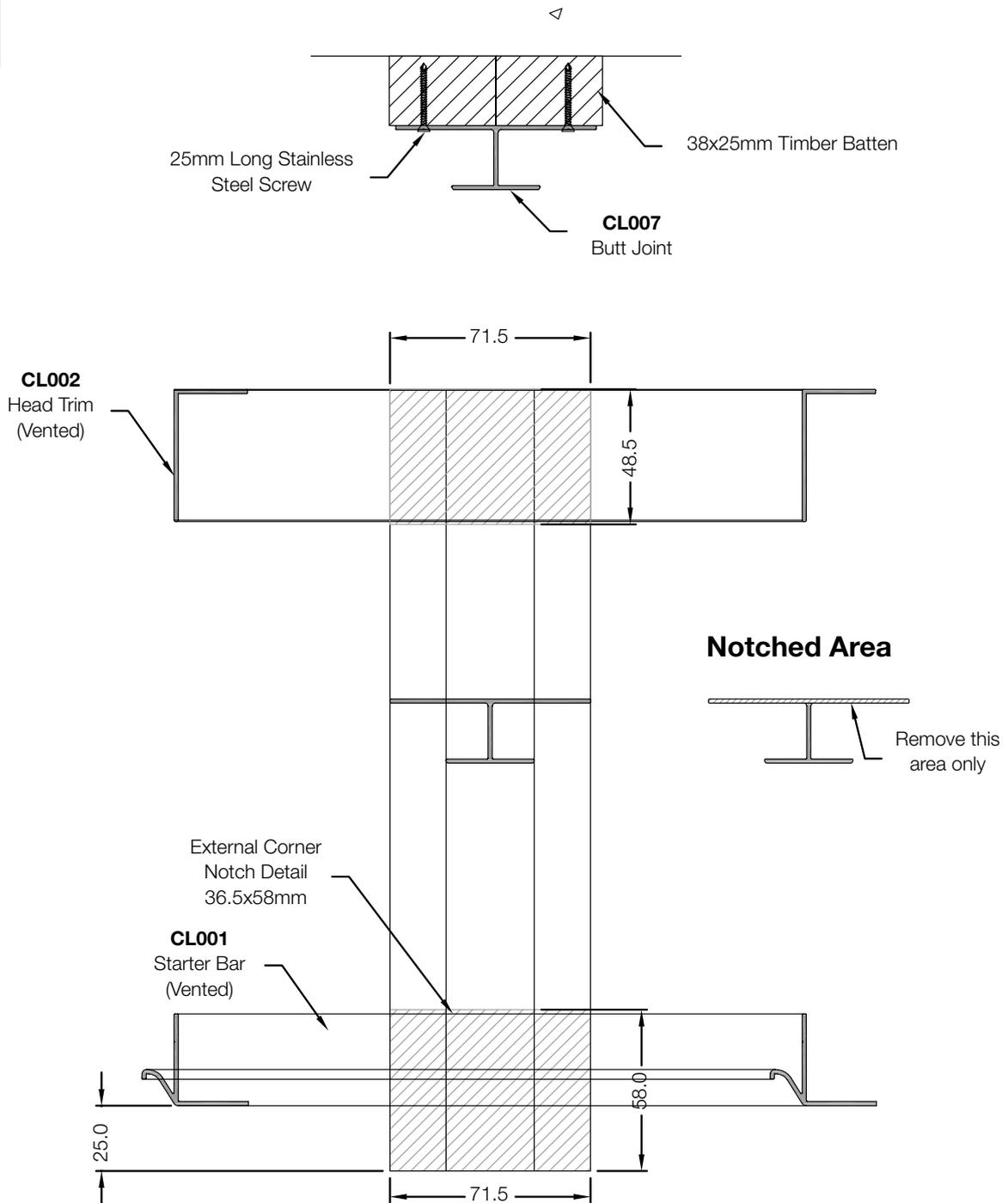
Where a butt joint is required, two vertical timbers are required to allow the butt joint to be fixed. Using stainless steel screws fix at 300mm centres. For the Butt Joint (CL007) to run full length the back section of the trim must be notched out where the Starter Bar (CL001) and Head Trim (CL002) run through.
