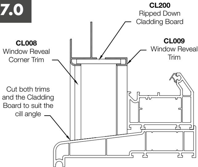
The Window Reveal Trims (CL008 & CL009) and the Cladding Board (CL200) will need cutting to suit the angle of the cill, this angle is dependent of the window which has been fitted and will vary from window to window.
