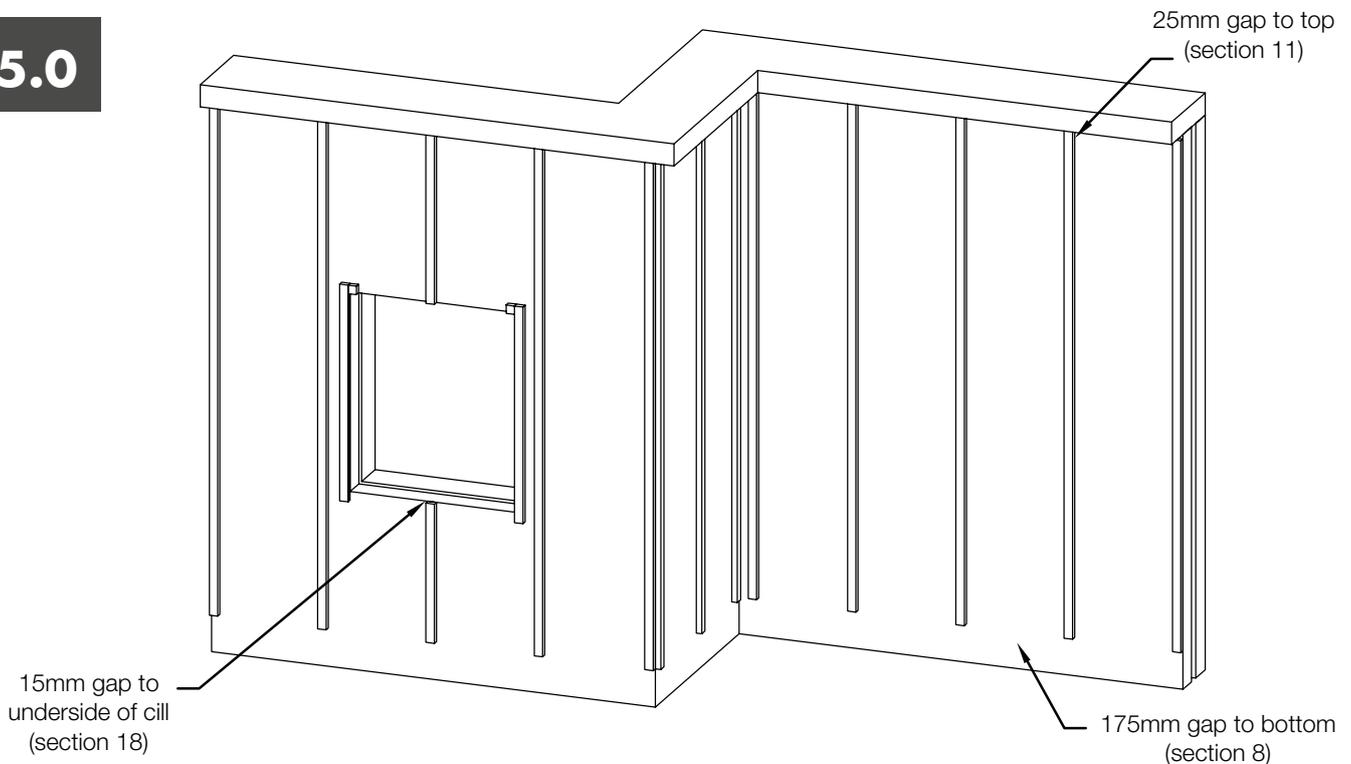
Position and fix the timber battens (38mm x 25mm) to the wall using stainless steel screws. Battens to run vertically starting at a minimum of 175mm from the bottom of the brickwork. Batten centres to be spaced at a maximum 500mm apart. The battens must finish 25mm short of the underside of a soffit and 15mm short of the underside of a window cill. (Refer to sections 8, 11 & 18 for more details).
