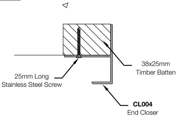
Locate the End Closer (CL004) onto the timber batten, fix using 25mm stainless steel screws. The End Closer (CL004) must be long enough to pass beyond the bottom of the first Cladding Board when fitted, the End Closer (CL004) should run 25mm past the bottom of the Starter Bar (CL001).
