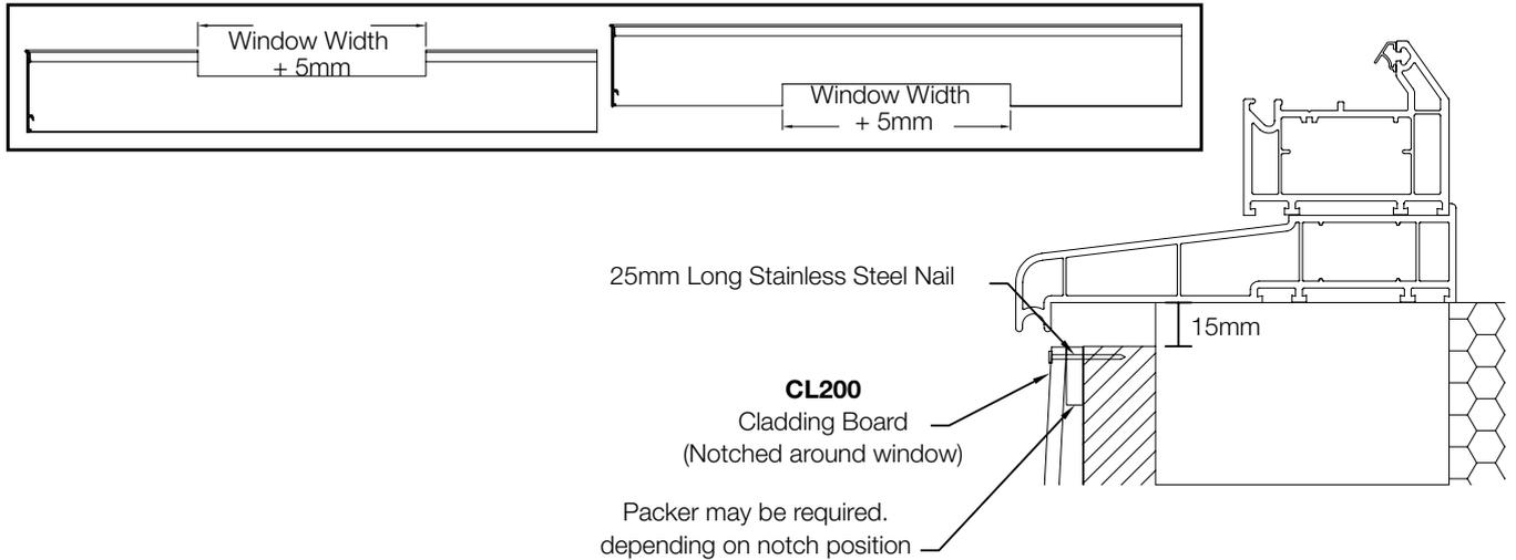
If cladding runs around a window, boards may need notching around the window at both the top and bottom. The size of the notch is dependent on the window size and where the stacked boards locate. Overleaf is an example of possible notching details for both over and under the window. A packer may be required behind the notched board to aid fixing.
