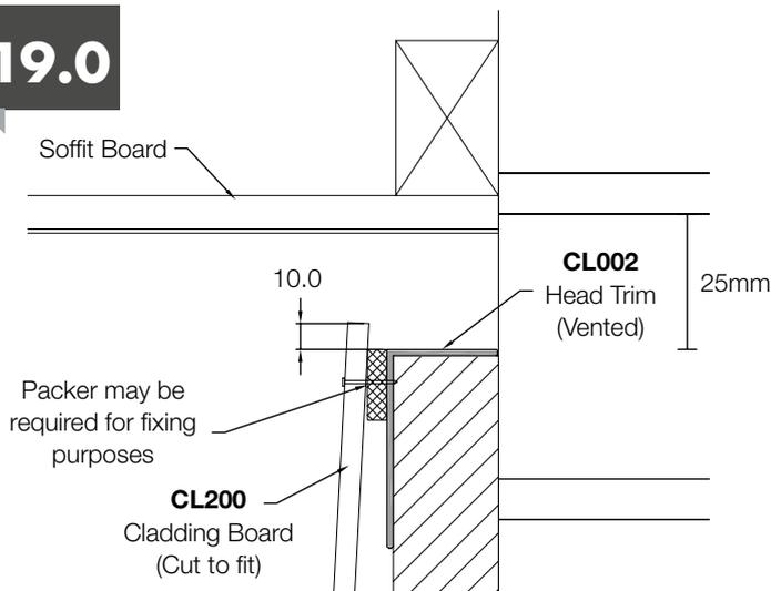
When fixing the final Cladding Boards at the top, run the board 10mm beyond the top of the timber. Depending upon how the board has been cut down to fit, a packer may be required to support the board when fixing.
