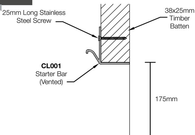
Once the window reveals have been completed fit the Starter Bar (CL001) to the bottom of the timbers, fix back to each batten as shown using 25mm stainless steel screws.
