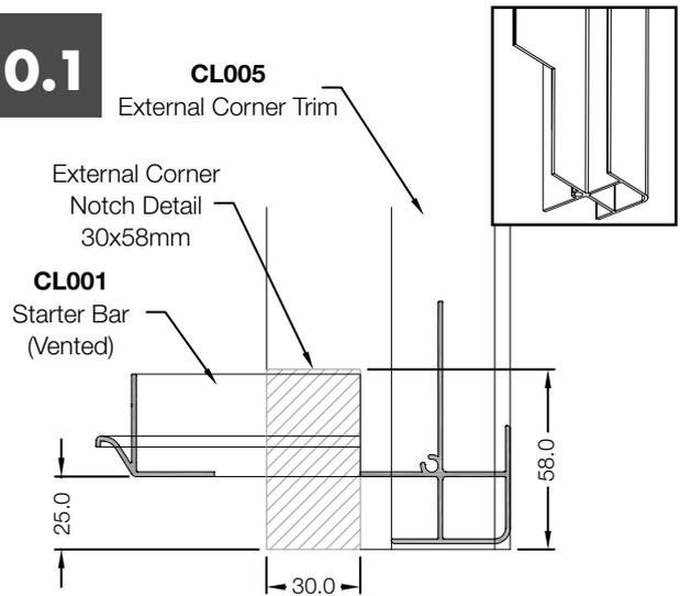
**Notching Details:-** To allow the Starter Bar (CL001) to run full length, notching is required on External Corner Trims (CL005). Cut away the section shown below.
