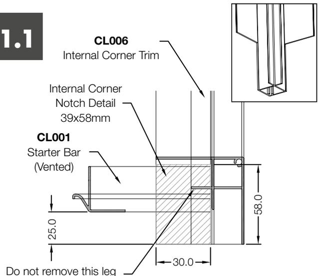
**Notching Details:-** To allow the Starter Bar (CL001) to run full length, notching is required on the Internal (CL006) Corner Trims. Cut away the section shown below.
