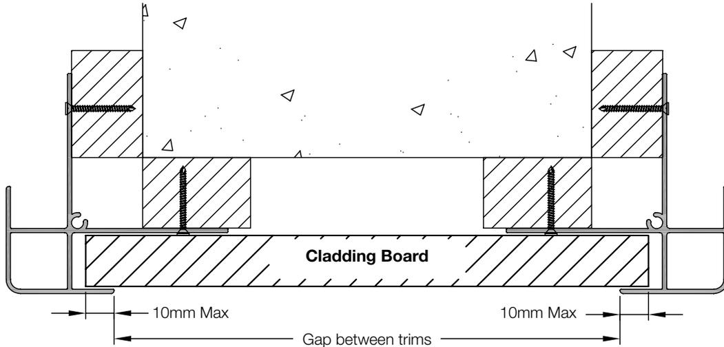
The Cladding Board cut length should be a maximum of 20mm longer (10mm per side) than the gap between the aluminium trims. Shorter board lengths may require the 10mm per side to be reduced to ease fitting and enable the board to shuffle into position rather than bend.
