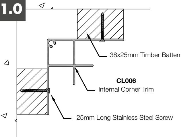
Fit corner trims to all Internal (CL006) and External Corners (CL005) as shown fixing with 25mm stainless steel screws at 300mm centres. The Corner Trims must pass beyond the bottom of the first Cladding Board when fitted, the Corner Trims should run 25mm past the bottom of the Starter Bar (CL001).
