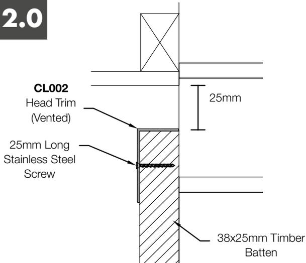
Fix Head Trim (CL002) to the top of the timber battens using 25mm stainless steel screws, fixing at each vertical timber batten.
