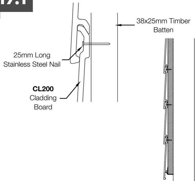
Once secure stack the next Cladding Board by hooking over the top lip which hides the fixings, as before fix back to the timbers through the top section of the Cladding Board. Continue this method until the cladding is complete.
