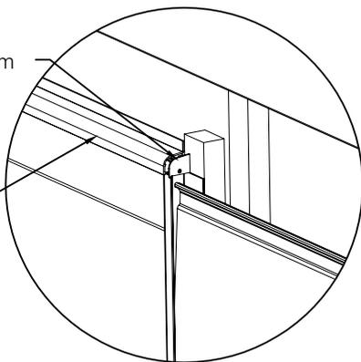
Window Head Trims (CL003) require to be capped off to create a neater finish, Window Head Trim End Closers (CL023) are available. Fix the End Closer to the Window Head Trim by screwing through the End Closer into the screw port in the aluminum extrusion using 4.5x16 pan head screws. (Touch up pens can be used to colour the screw ends where they will not be covered by boards).
