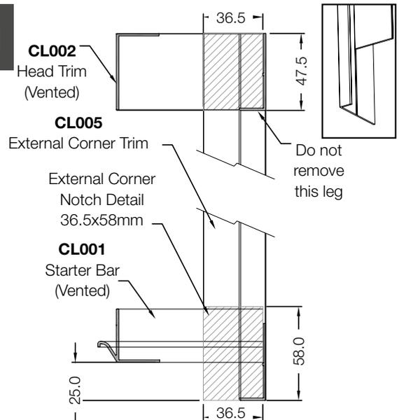
**End Closer Notching Details:-** To allow the Starter Bar (CL001) and Head Trim (CL002) to run full length, notching is required on the End Closer (CL004)
