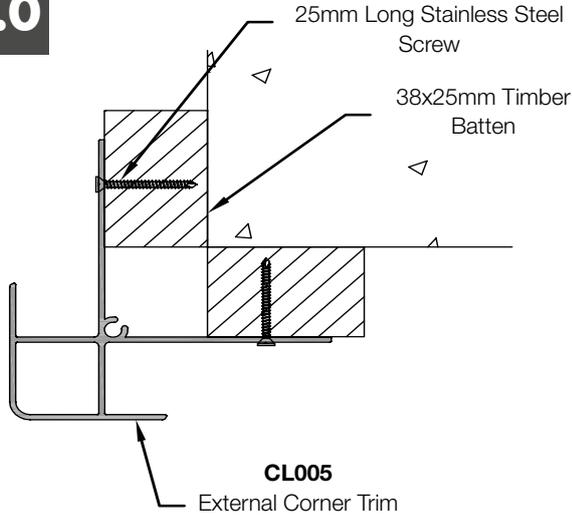
Fit corner trims to all Internal (CL006) and External Corners (CL005) as shown fixing with 25mm stainless steel screws at 300mm centres. The Corner Trims must pass beyond the bottom of the first Cladding Board when fitted, the Corner Trims should run 25mm past the bottom of the Starter Bar (CL001).
