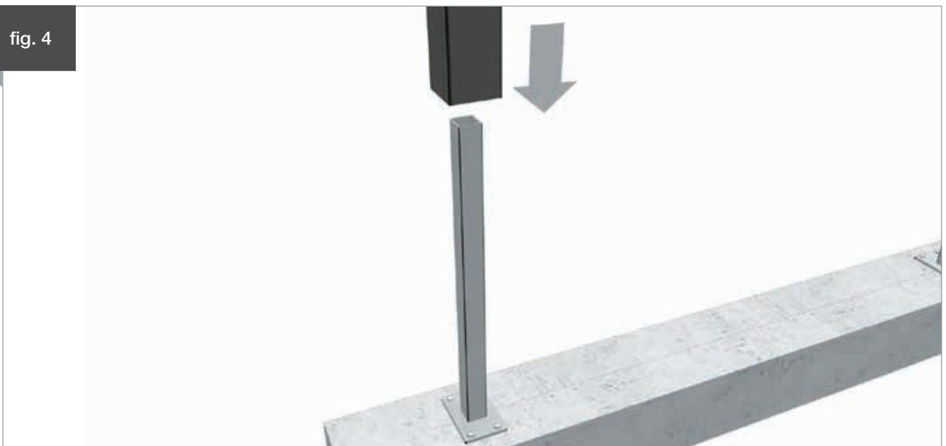
Slide the fence post over the steel insert.
