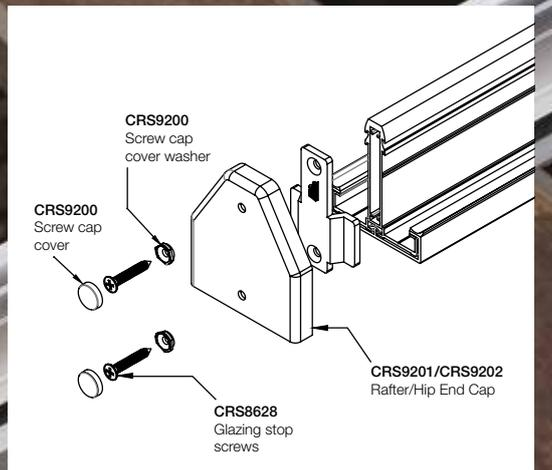
It is advisable to partially fit the glazing stops and end caps as shown (right) before fixing rafters to the ring beam. **Install the glazing stop screws to approx. half their length, do not install screw cap covers at this point.** You can then proceed to loosely secure the side rafters to the ring beam using the threaded studs located down the ring beam.
