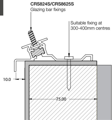
Ensure correct amount of glazing bar fixing studs are slid into the ring beam before any fixing commences. Position the ring beam so an equal overhang is achieved around perimeter and fix using suitable 5-6mm fixings at 300-400mm centres (starting and ending 100mm away from internal corner of the ring beam).
