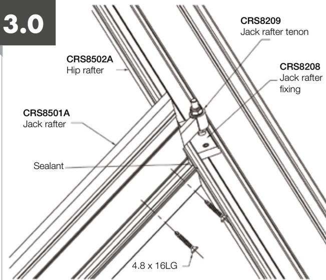
Locate the jack rafter tenon onto the jack rafter fixing bolt and adjust the lower nut to align gaskets, before tightening the the top nut.
