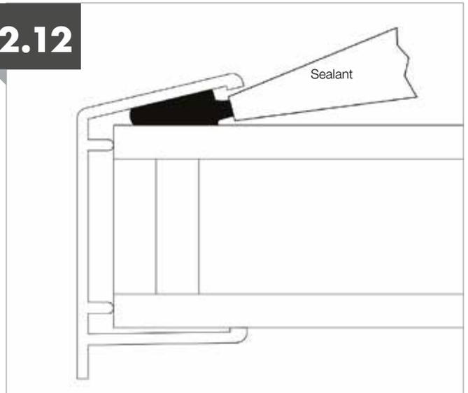
Fit the glazing end closures to the glass and run a bead of sealant between the profile and top pane of glass as shown above. **Only** use a suitable sealant with self cleaning glass. Soudal SMX 506 is recommended (available from Eurocell branches).
