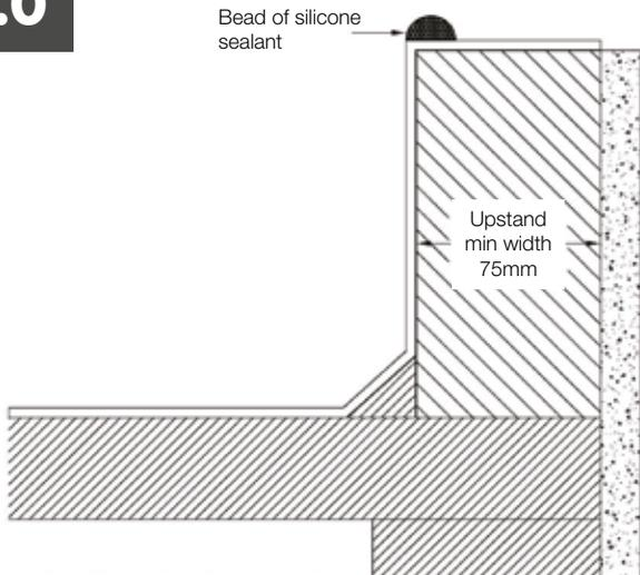
Ensure the kerb is clean and free from debris, then run a silicone bead around the external edge as shown above.
