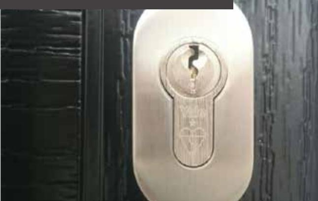
These should be fitted using the screws provided and pilot drilled using a 2mm drill bit. Never drill more than 10mm into the door leaf as damage to the lock can occur if you drill deeper.
