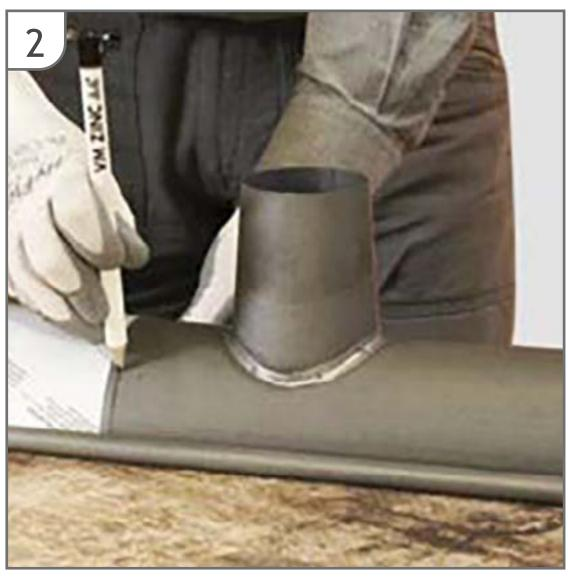
Cut the running outlet to the required length, starting from the rolled front edge.
