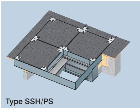
Gatic Parade 2 hour fire rated Multispan Stainless Steel Recessed Covers and Frames with Removable Beams, galvanised baseplate and reinforcement, double sealed with socket head securing bolts/unsealed with blanking bolts\* to suit a pit clear opening of ..... x ..... suitable for Medium Duty – 5 tonne slow moving pneumatic wheel load Stainless Steel Grade 304/316\* Type **SSH/PS**.
