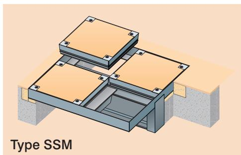
Gatic Parade 2 hour fire rated Multispan Stainless Steel Recessed Covers and Frames with Removable Beams, galvanised baseplate and reinforcement, double sealed with socket head securing bolts/unsealed with blanking bolts\* to suit a pit clear opening of ..... x ..... suitable for Medium Light Duty – 3 tonne slow moving pneumatic wheel load Stainless Steel Grade 304/316\* Type SSM
