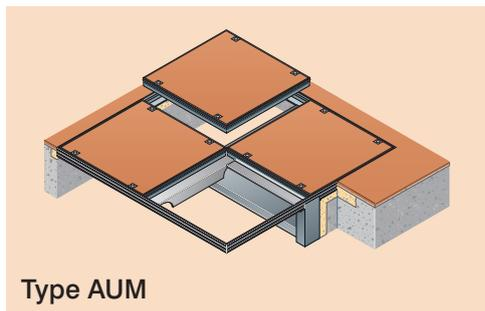
Gatic Parade 2 hour fire rated Multispan Aluminium Recessed Covers and Frames with Removable Beams aluminium/brass\* edging, top edge dirt seal, mechanically jointed corners, galvanised baseplate and reinforcement, double sealed with socket head securing bolts/unsealed with blanking bolts\* to suit a pit clear opening of ..... x ..... suitable for Medium Light Duty – 3 tonne slow moving pneumatic wheel load Type AUM or AUM/B\*
