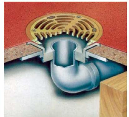
Watertight drainage in a vinyl covered timber floor.
