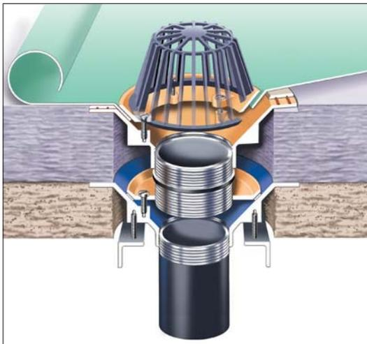
WC224Z roof outlet with WG102 underdeck clamp and WT103 threaded pipework adaptor, in a warm roof with single ply membrane.
