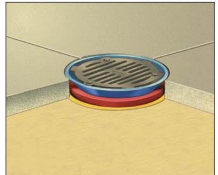
Fit dome/grating using height adjustment where applicable to ensure grating is flush with roof finish. Apply roof finish around grating.
