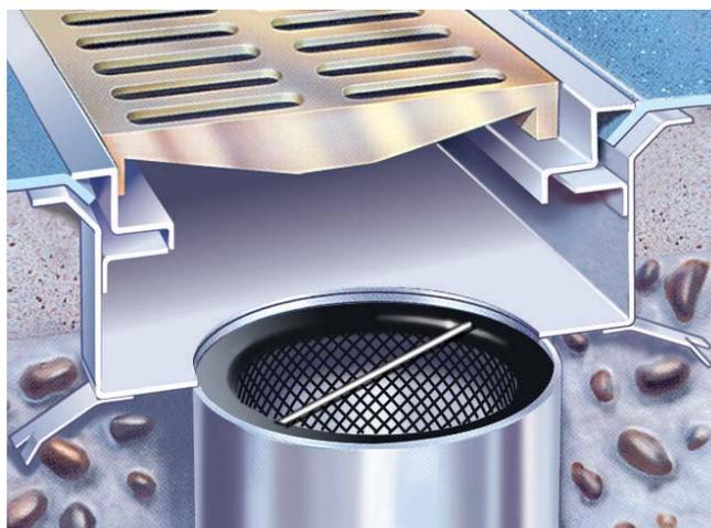
*Channel profile SVF ensures watertight connection when used with flexible sheet floor covering such as vinyl.*
