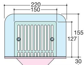
Wade offers a range of parapet outlets often used with downspout nozzles as shown below. A membrane clamping collar, of stainless steel is supplied with stainless steel grating versions. This allows the grating to be removed, for maintenance purposes, without disturbing the membrane. Versions with aluminum grating use the grating as a membrane clamp.
