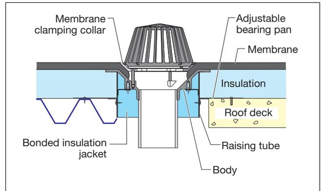
On site the raising tube can be easily slide-positioned through the bearing pan to suit the insulation thickness. When the required height is achieved, the tube is secured to the bearing pan using the self-tapping screws provided. The bearing pan is designed to be fixed to the deck/slab, so an underdeck clamp is not necessary.
