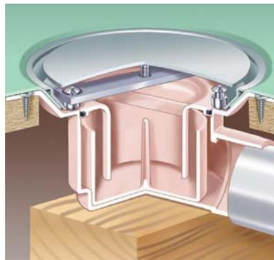
Watertight trapped drainage in a vinyl covered timber floor.
