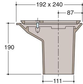
Outlet spigot conforms to BS416 / DIN19522
