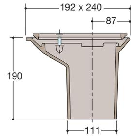
Outlet spigot conforms to BS416 / DIN19522
