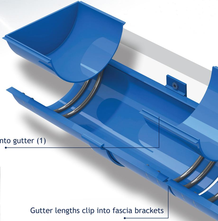
Snap Fix union clips into gutter (1)
