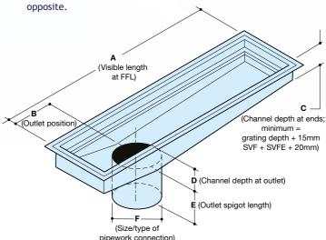
To suit particular applications channel can be custom made in grade 304 or 316, with or without fall, with a combination of different profiles, on the same or opposite side, with non standard profiles including deep invert, 'V' bottom and heavy duty versions. Please contact our Technical Services Department for details.
