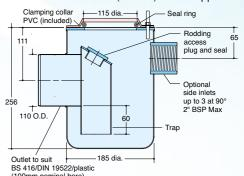
Non-trapped - Stainless steel grade 304 (for grade 316 add suffix 'M' to Spec. Code)
