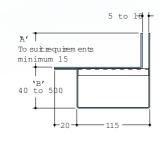
Rodding access - 140mm square access covers are fitted over the outlets, as standard; these may be recessed to accept flooring material.
