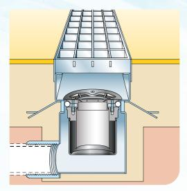
NE channel and SS5135B5 grating, shown with Q21 style 2" BSP horizontal side outlet and U1404 removable bottle trap.
