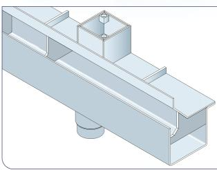
Spec. Code: TDN 'D' → -50-Generally 10 25 to 75 'C' 0 to 20 Optional horizontal 2" BSP female outlet 'B' 75 to 110 2" BSP female outlet with T1702 adaptor to 50mm plastic pipe
