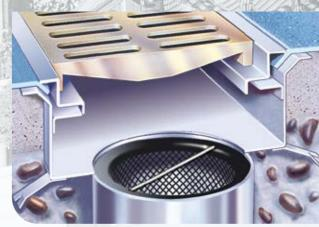
Typical installation in a vinyl covered floor SN12230 grating with SVFB channel. Channel profile SVF ensures watertight connection when used with flexible sheet material such as vinyl flooring. Suffix 'B' on channel Spec. Code denotes filter bucket.
