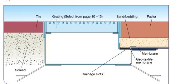
Single secondary drainage (SSD) with channel profile NE
