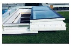
Starglaze units come ready to fit directly to the roof deck with either splayed or vertical upstands. Splayed upstands deliver a more even distribution of natural light, while vertical upstands have the benefit of maximising the quantity of light being brought into a property.
