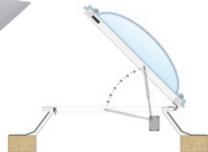
Access hatch on 150mm splayed PVC upstand
