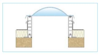
MK2 vertical unventilated PVC kerb/upstand fitted direct to roof deck
