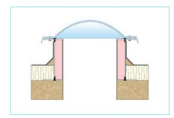
MK3 vertical unventilated thermally broken aluminum PVC kerb/upstand
