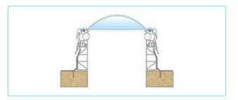
MK1 unventilated PVC kerb/upstand fitted direct to roof deck
