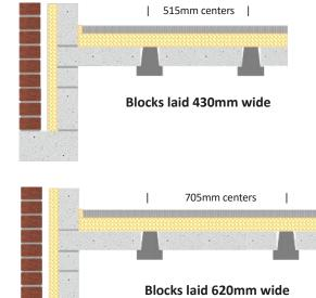
**Note:** The center widths are approximate and based on a typical 150mm deep T-beam profile which may vary depending on beam type.
